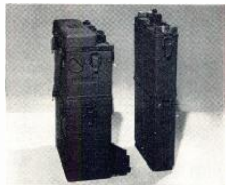
Comparison in size between the World War II walkie-talkie (left) and the new AN/PRC-10 model developed by RCA. The new unit is approximately half the size of the older unit and has greater coverage.
