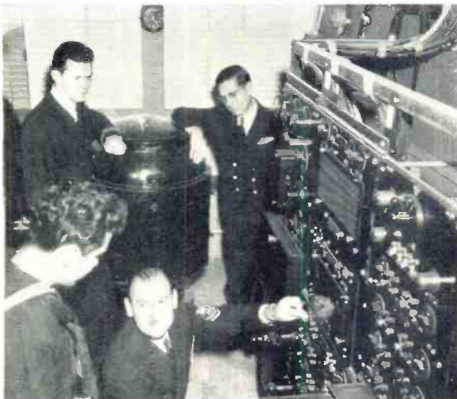
The gyro room at the Naval Reserve Training Center in Albuquerque, New Mexico showing the Sperry gyro compass and the repeater panel board. Shown in the photograph standing (from l. to r.) are A. Garcia, Lt. E. W. King, and C. R. Stanello. K. E. Langley, seated at controls, demonstrates unit's operation.
