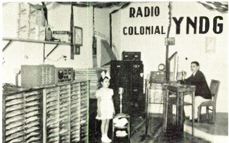
YNDG, 5.995, Radio Colonial, Leon, Nicaragua, uses a Hallcrafters BC-610E. Since this photograph was taken the station's power has been increased to 1 kw. and additional equipment has been added. Dennis E. Gallo is the manager of this outlet.
