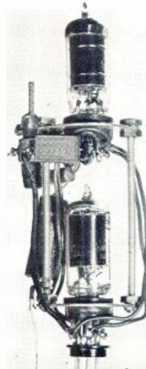
Fig. 1. Over-all view of Turret Booster.
