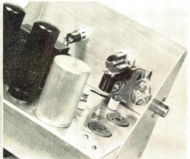
(Left) Bottom view of transmitter. (Right) Rear view of transmitter portion with tubes removed. Either APC type trimmer condensers can be used for C 10 or C 11 , as indicated in the parts list, or ceramic type condensers, shown in the author's rig, can be used.
