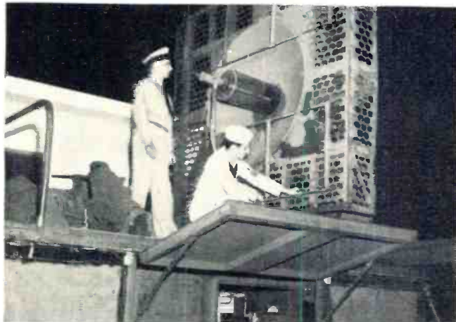
Members of the Organized Surface Division 8-73 at the Naval and Marine Corps Reserve Training Center in Corpus Christi, Texas assist in the conversion of an Army radar unit to a hurricane warning radar unit. This instrument, which is the property of the A & I College in Kingsville, Texas, is being maintained by the Central Power and Light Company and is in operation at the Clift Maus Airport in Corpus Christi, Texas.
