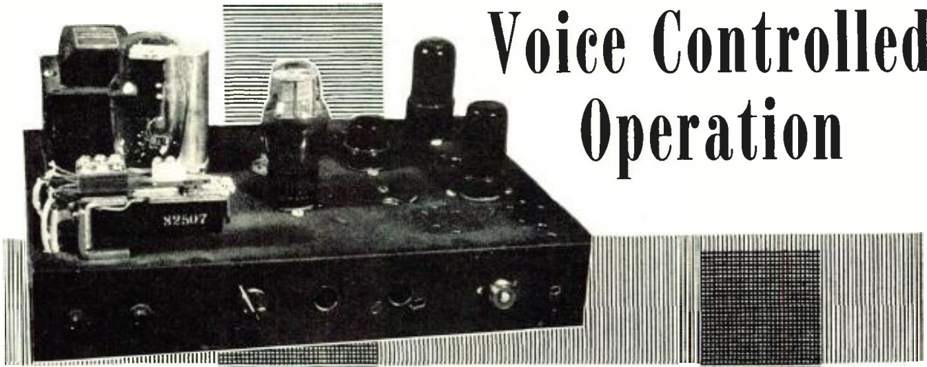
Over-all view of a voice control unit which can be added to any transmitter.
