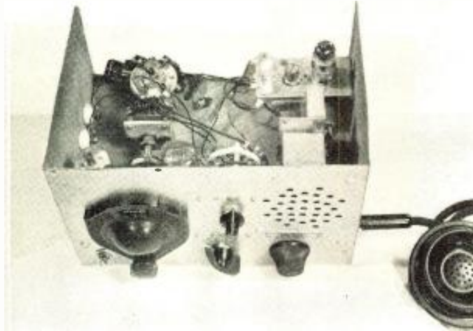
Top view of transceiver. Toggle switch, not included in schematic, shown on front panel is connected in power supply circuit.
